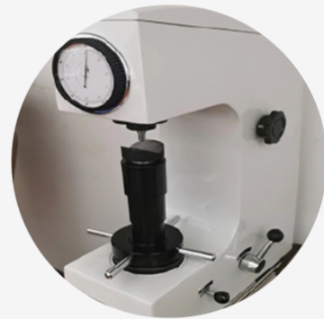
ROCKWELL HARDNESS MACHINE
